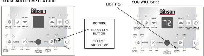
Note: Fan starts at High Speed and adjusts to a slower speed as the room temperature dictates. For example if the room doesn't get too warm, it will stay at the slowest speed. If the room temperature rises quickly, such as a door being opened, it will automatically go to the highest speed. The fan speeds will re-adjust back to the slowest speed as the room returns to the original set temperature. Press the fan button to adjust the fan speed manually.
